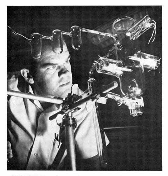
A Sandia advance in the field of thermionic conversion may pave the way for a breakthrough in space power systems. Provided certain heat - containing materials problems can be solved, the use of chemically vapor deposited (CVD) rhenium on thermionic emitter and collection plates (electrodes) should make possible nuclear space power generators that are twice as efficient as the SNAP generators now in use.
